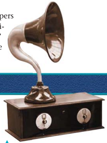
By 1930, 40 percent of U.S. households had radios, like this 1927 Cosser three-valve Melody Maker.
